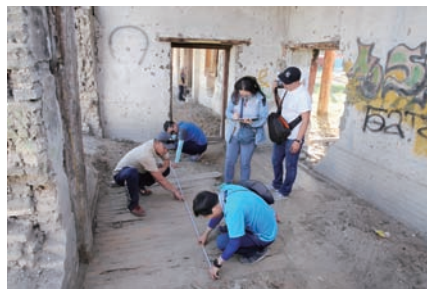
Measuring the wooden floor of the side room at the front of the building
